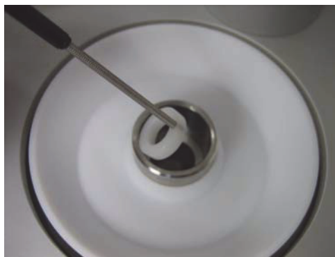
Figure 4. Removing the reference cell lid over the reference cell port.
